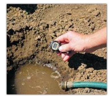
All of the water must drain away within 8-12 hours after the second filling (or at a rate of 1 to 2 inches per hour.) to result in the survival of your tree.
